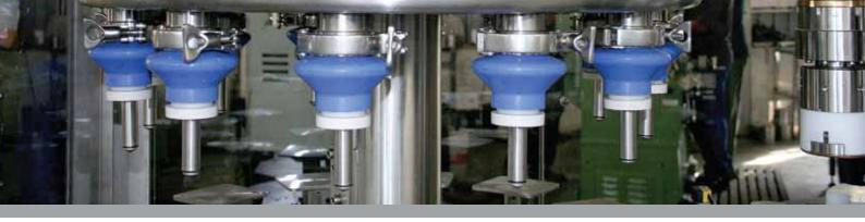
Filtec Automation offers a range of **Rotary Level Filler Cappers**, to fill free flowing low viscosity products such as milk, water, beverages, cordials, vinegars etc. The Filler can handle a large range of glass and plastic bottle sizes.
